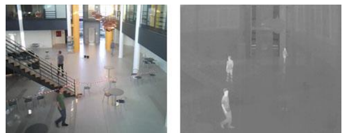
Fig. 2. A scene captured using visible and thermal camera [18]
