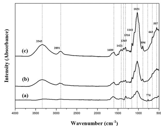
Fig. 2. Characterization of WRMA and LCNFs. The FTIR-ATR pattern of (a) WRMA; (b) LCNF-1h; (c) LCNF-3h
