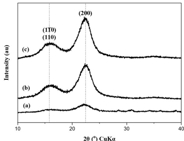
Fig. 1. Characterization of WRMA and LCNFs. The XRD pattern of (a) WRMA; (b) LCNF-1h; (c) LCNF-3h
