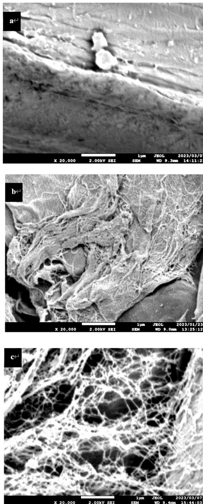
Fig. 3. FE-SEM images of WRMA and LCNFs of (a) WRMA; (b) LCNF-1h; and (c) LCNF-3h
