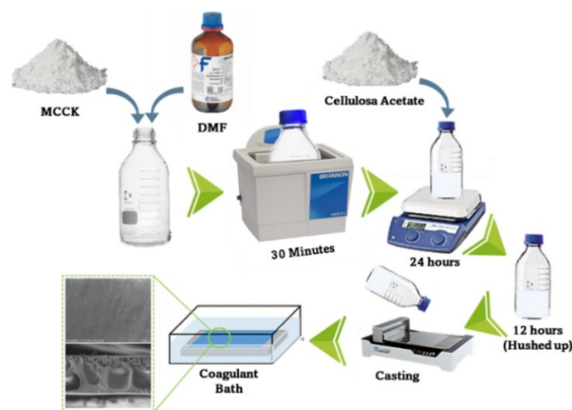
Fig. 1. Process for making cellulose acetate/MCC composite membranes
