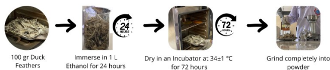
Fig. 1. Pre-treatment process to remove all types of contaminants, both organic and inorganic compounds
