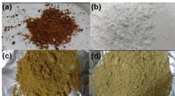
Fig.1. Spray drying powder results: (a) Propolis without encapsulation; (b) maltodextrin-gum Arabic; (c) SDMP rough type; and (d) SDMP smooth type
