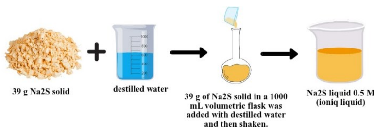
Fig. 2. Preparation of ionic liquid solvent for extraction
