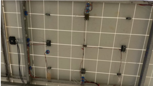
Fig. 2. Installation of PT100 RTD on PV module
